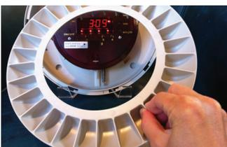
Place the pill tray back into the base. Wait for the alarm to go off. When it does, you will see the medication wheel turn and hear the alarm ring. Let it ring for the full three minutes. At the end of the time, you should see the large LED light come on. This means it is sending the notification signal.
