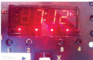
Set your dispense alarm times. Medication can be dispensed up to 4 times a day. Set only the number of alarms you need. Leave the remaining alarms deactivated to avoid overdosing. To set the alarms, press and hold the desired alarm button (1-4). You should see the time change on the clock panel. Continue to hold the alarm set button as you change the time with the Hour, Min, and AM-PM buttons.
