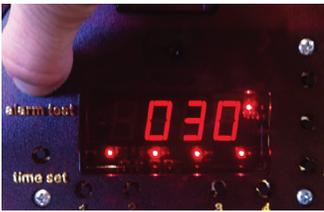
Reset the notification time back to :30 or desired time by pressing and holding the Alarm Test button to display the current setting of :03 and using the MIN button to adjust the time back to :30 minutes (or desired time).
