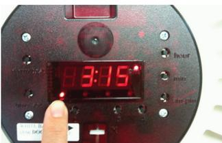
Test the dispenser's ability to generate a medication dispenser alert. Press and hold the ALARM Test button while you adjust the number on the clock from :30 to :03 minutes with the MIN button. This reduces the amount of time it takes to report an alert. Using alarm button 1, set ALARM 1 for a time 5 minutes past the displayed time on the clock. Once the alarm is set, make sure it is active by verifying the LED light is on above ALARM 1.
