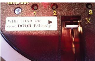
Make sure the white bar is in the locked position next to the clock.
