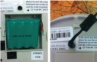
On the back of the dispenser, locate back-up battery compartment door. Open and insert the battery by plugging into small hole. To verify proper installation, the color light will blink on the front panel.
