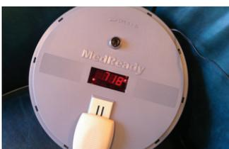
Place the lid on the medication dispenser. Make sure the door on the lid is closed as you place the lid on the base. Lock the lid with the key, remove the key, and return it to its secure location.
