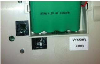
Connect the supplied phone cord to either of the phone jacks on the bottom of the dispenser. Connect the other end of the cord to a landline telephone jack.
