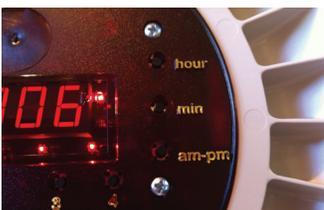
Before activating, make sure all alarms are turned off and the white T-bar is pushed all the way up. Then press and hold the AM-PM button on the dispenser for about 5 seconds or until you see the large red LED light come on. When this lights up, it means the dispenser is connecting with the server.
