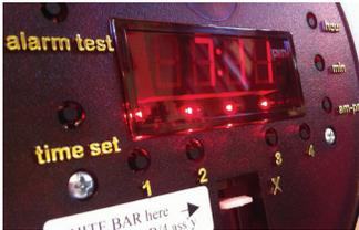
Set the main time on the clock to the current time by pressing and holding the Time Set button while you change the time with the Hour, Minute, and AM-PM buttons. NOTE: AM and PM are indicated by the red light found under the letters "PM." If the light is on, that means the time is a PM time.
