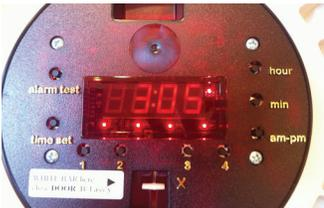
Turn the dispenser back over and deactivate alarms 1,2,3, and 4 by pressing and holding the numbered buttons one at a time. The red light above each button will turn off.
